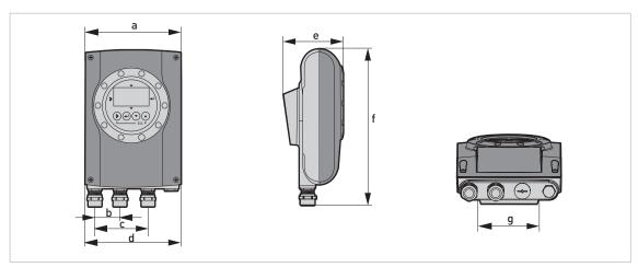
Figure 2-2: Dimensions of compact version
