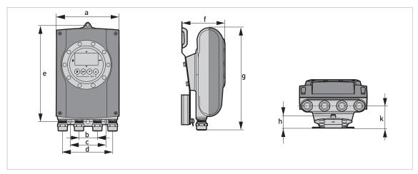
Figure 2-1: Dimensions of wall version
