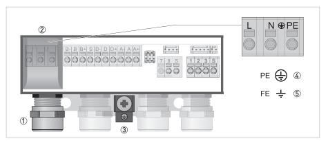
Figure 4-4: Terminal compartment for power
