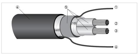
Figure 4-1: Construction of signal cable A
