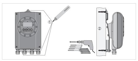
Figure 3-1: Mounting of the wall housing
